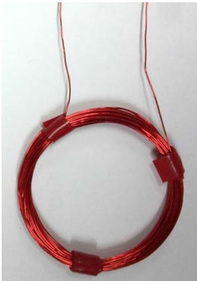
**Depending on the size, the turn, the thickness of the wire and the diameter, the transmitting Frequency becomes different.**
